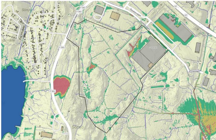
Figur 13. Skyfallsanalys (flash flood) i Scalgo Live. 50 mm. Grönt=0-30 cm, gult 30-50cm, rött>50 cm
